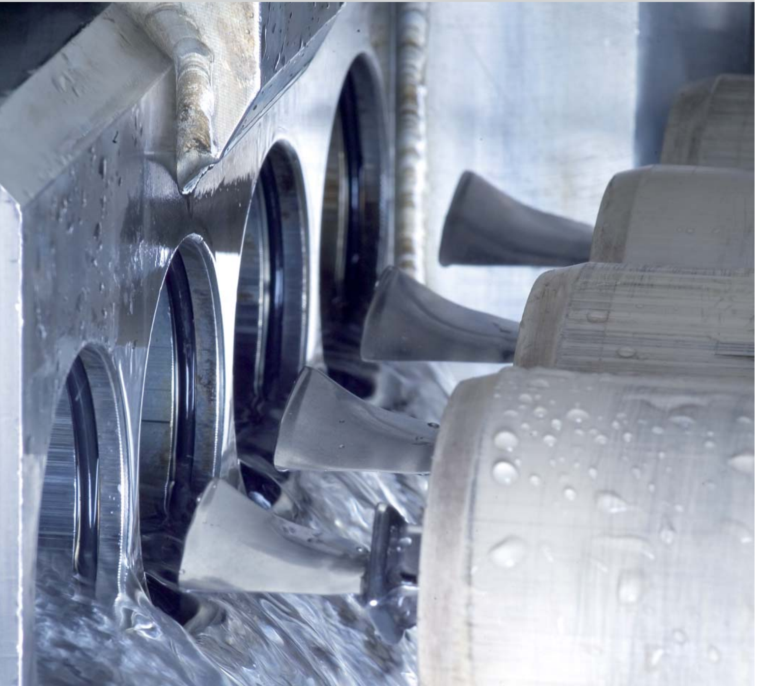
Detail showing ECM of compressor airfoils
