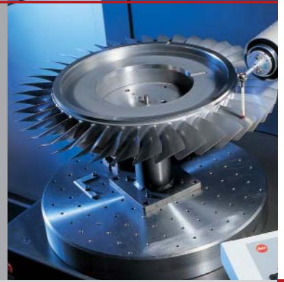
CMM measuring of a Blisk/IBR
