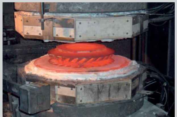
Isothermally forged Blisk from Ti6246
