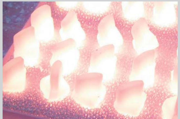
Compressor blades of TiAl during solution annealing
