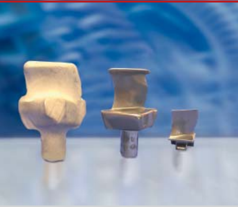
Process steps of a TiAl compressor blade
