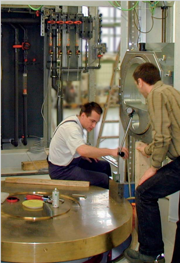
Assembly of an ECM machine
